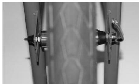
6. Tighten the quick release lever.
