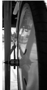
5. Pull the wheel to the front of the bicycle so that the chain is running firmly but not too tight.
